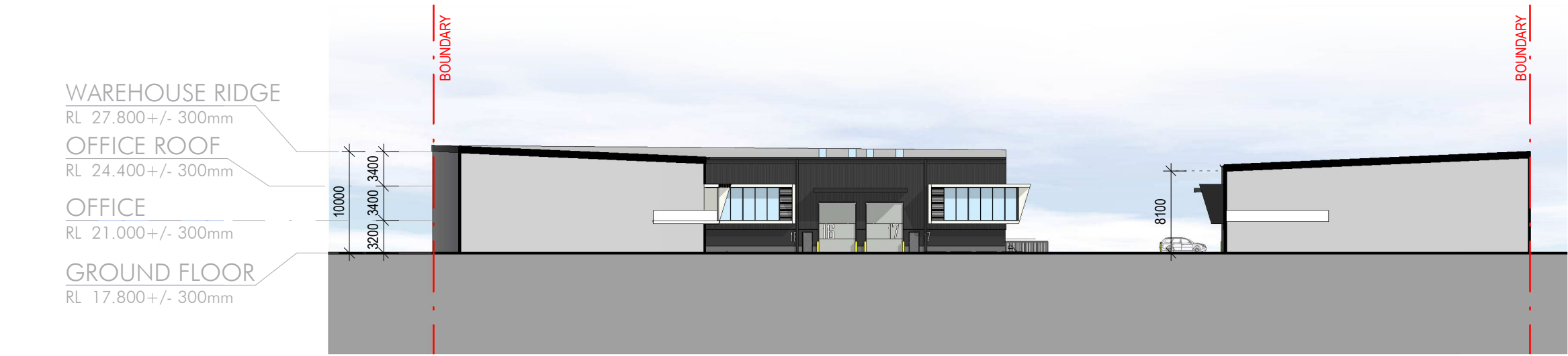
3 South Elevation - Warehouse 1 Elevation/Section & Warehouse 2 Section 1:500
